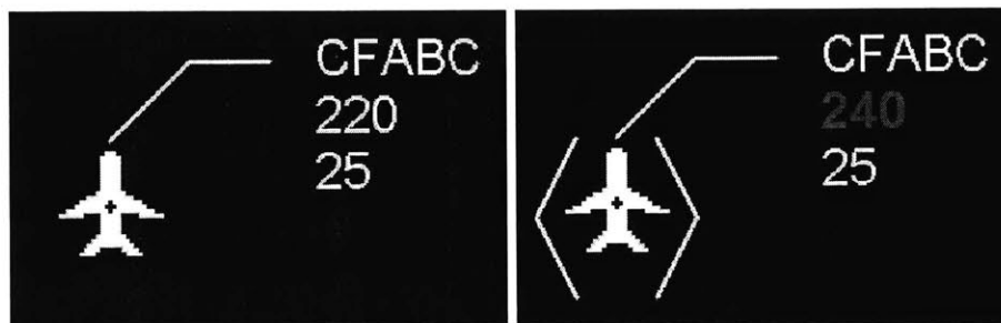
Figure 2.8: CAATS Display Symbology for Conforming (left) & Non-Conforming (right) Aircraft [adapted from Pelletier (2002)]
