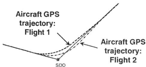
Figure 5.17: Comparison Between Lateral Transition Trajectories for Flight Tests 1 & 2
