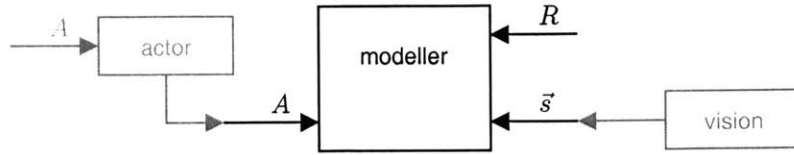
Figure 6-4: A position-trigger modeller tries to find an association between a state parameter \vec{s} , an actor’s activation A , and reward R . The goal is to determine a region of the space of \vec{s} (a context) which leads to the actor being activated (triggering the execution of an action).
