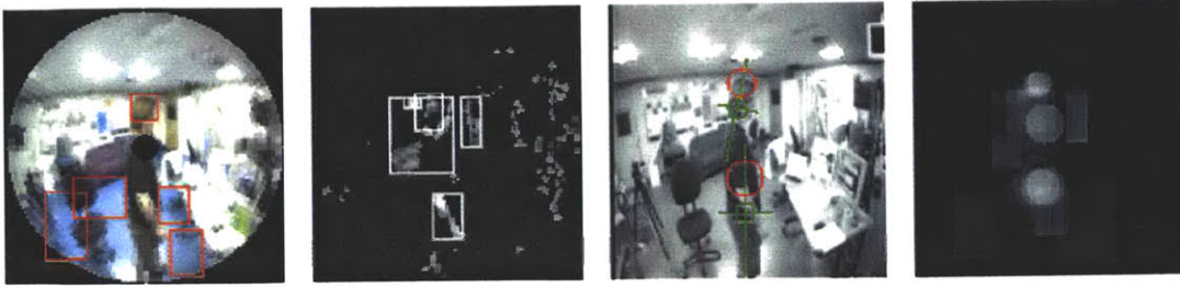
Figure 4-7: Saliency and attention processing while looking at a walking person. One frame each from the three saliency filters (vividness, skin tone, and motion) and the attention system is shown. The vividness filter picks out parts of the blue floor. The skin tone filter picks out the person’s arm and hair, a door, and the couch. The motion detector highlights picks out two targets on the person’s body. The regions chosen by the filters are weighted together by the attention mechanism, which favors the motion detector.
