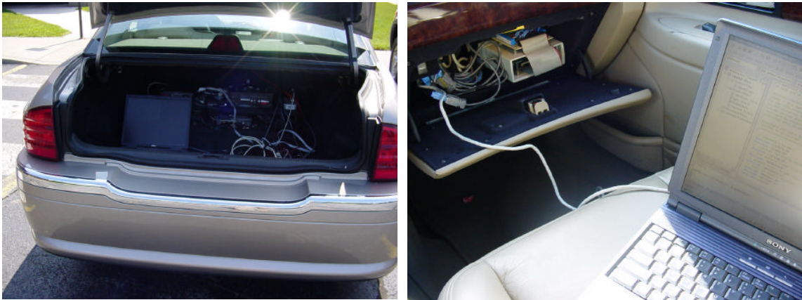
Figure 4-1: Lincoln LS Setup- a central processing unit and a warning system unit
