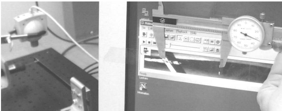
Figure 3-12: Data measurement from camera output. The data presented in this section were all recorded using calipers to estimate position on the computer screen, as depicted above. Note that students taking 2.003 simply estimate position with respect to a scale mounted above the cantilever (and also recorded in the video). The caliper measurements are simply more precise, despite the effects of parallax.
