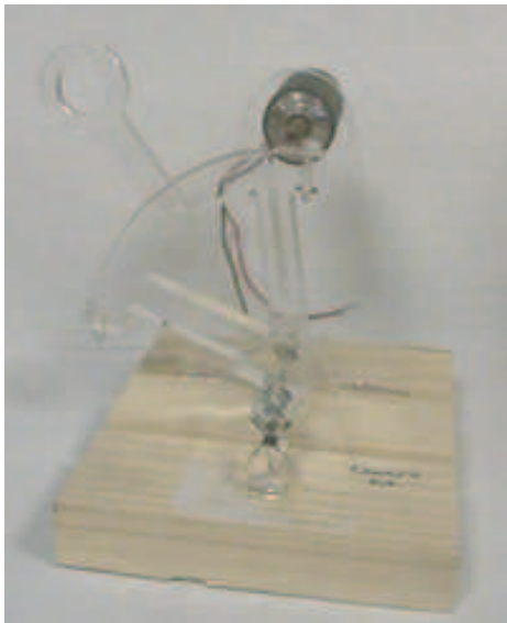
Figure 2-15: The Stanford haptic paddle [152] with step response data [169]. Students in Stanford class ME161 were asked to tune the haptic paddle system to obtain a lightly damped response. In the representative data shown above, the haptic paddle “sticks” due to Coulomb friction, causing the actual data to vary noticeably from an ideal, 2nd-order response.
