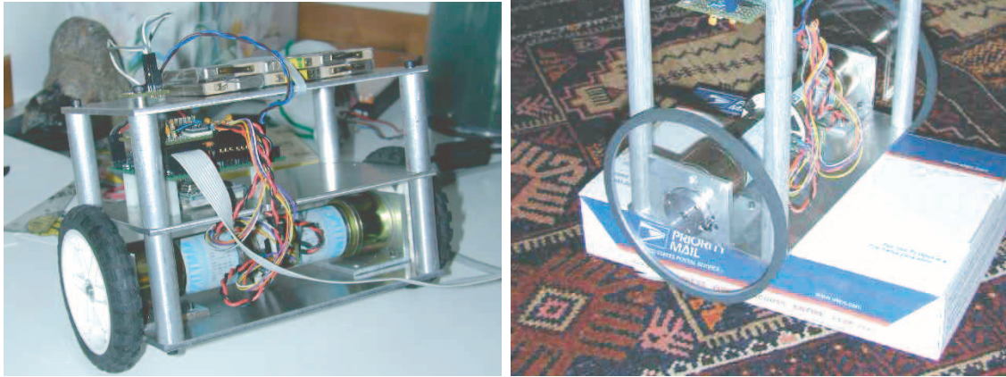
Figure 2-12: “GyroBot” two-wheeled IP platform robot. Created by Larry Barello. The taller version of this robot (at right) is reported to be more stable than the earlier prototype (left). ( http://www.barello.net/Robots/gyrobot/index.htm )
