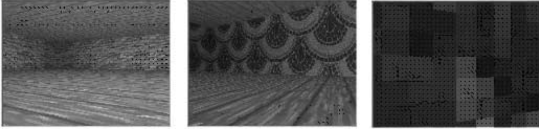
Figure 4-2: The virtual robot roaming through open rooms. The left frame shows the robot approaching the corner of the room with stone brick walls. The middle frame shows the mosaic pattern walls. The right picture shows the robot's field of view after colliding into the mosaic wall. Notice that all the optical flow vectors and their respective patch centers are visible.
