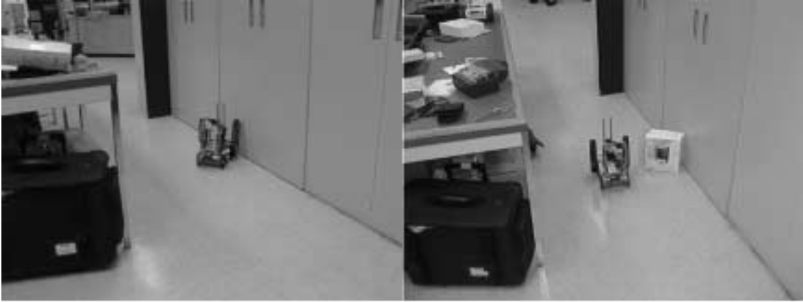
Figure 4-8: The robot driving between a table and cabinet. On the left, the robot collides into the lightly textured cabinet. On the right, the robot is able to avoid the cabinet after an additional textured obstacle is placed in its way.
