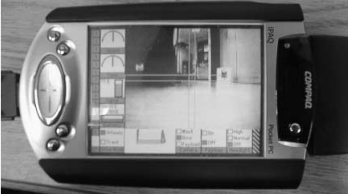
Figure 2-2: An active Operator Control Unit (OCU).
