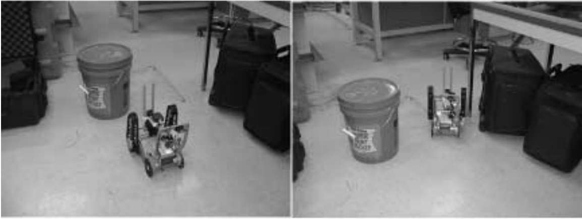
Figure 4-4: The robot driving between a bucket and a table. The robot approaches the bucket (left figure), turns right to avoid the bucket, and drives between the bucket and the table leg (right figure).
