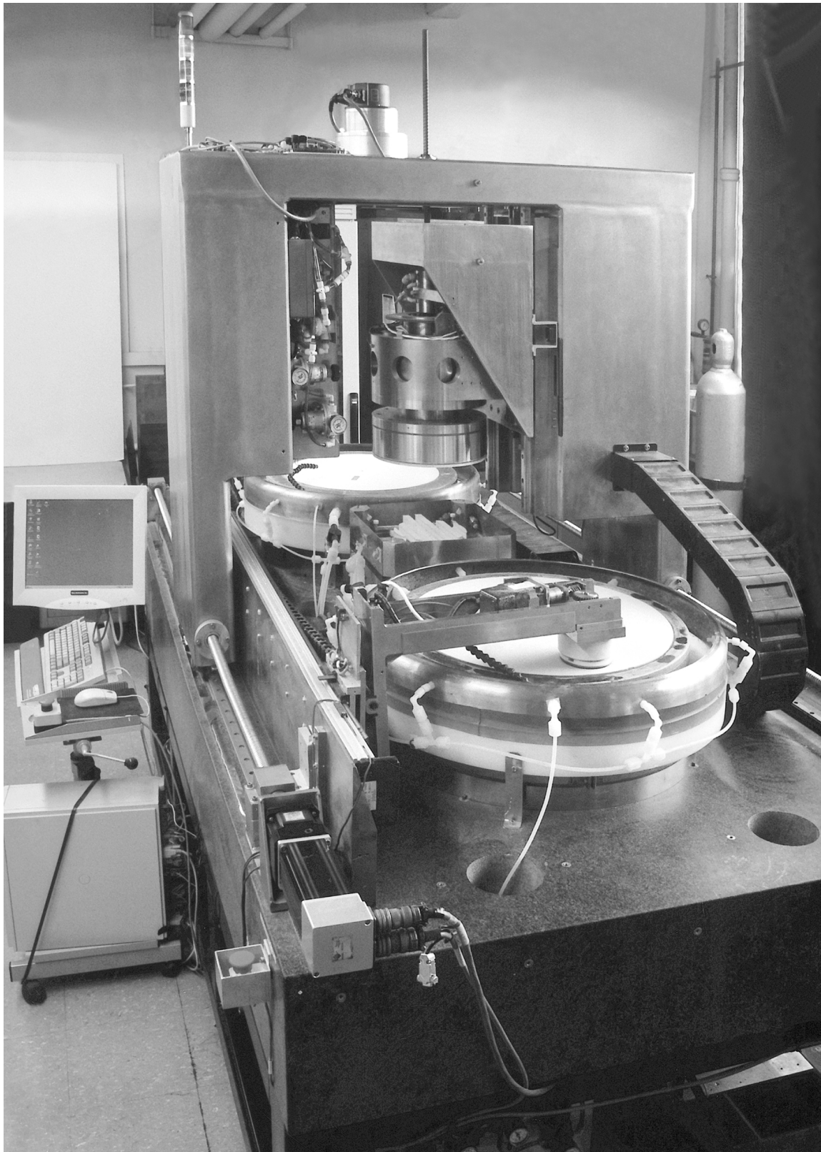
Figure 6-2: Photograph of the fabricated MIT CMP Platform
