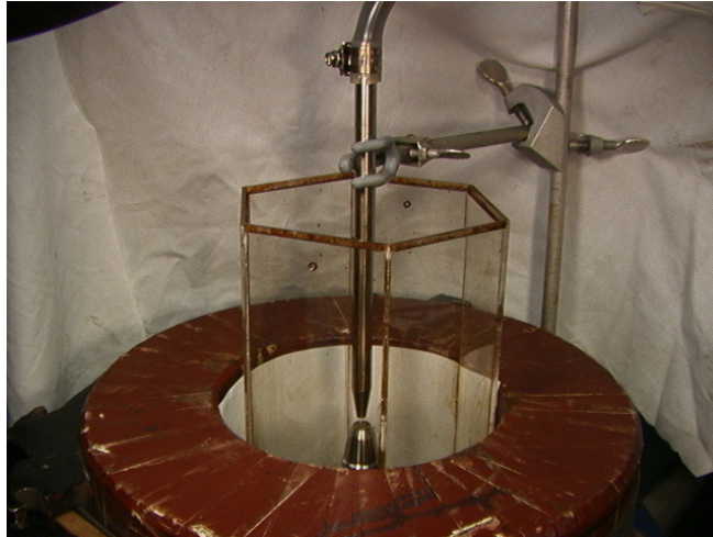
Figure 4.18: The test cell is placed inside the vertical magnetic field created by the electromagnetic. The ferrofluid jet is aligned with the magnetic field while the resulting radial sheet flow is perpendicular to the magnetic field.
