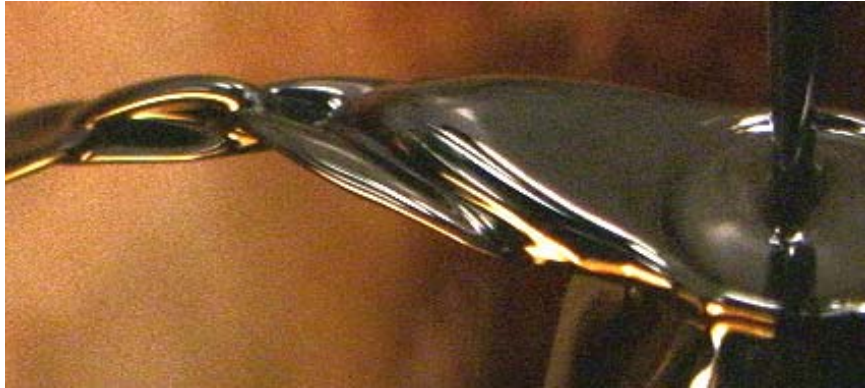
Figure 4.10: A close-up view of a ferrofluid chain at the tip of a lenticular ferrofluid sheet.
