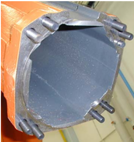
Figure 4.3 Existing Coupling Features on Arm Figure 4.4 Existing Coupling Features on Wrist
