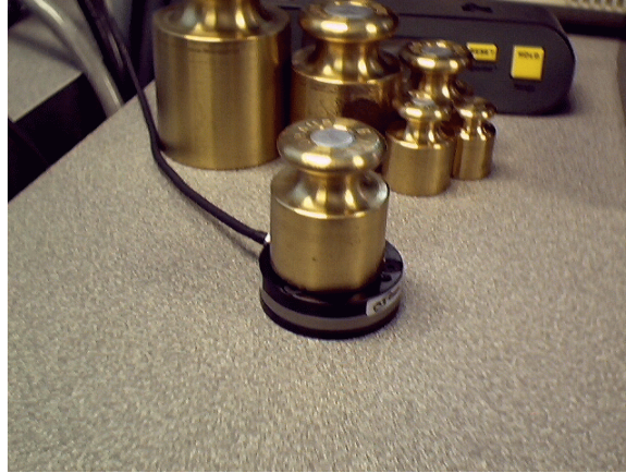
Figure 3-5: The Mini-40 6-axis force/torque sensor is shown above, where we have used small standard brass masses to test the Z-axis calibration.
