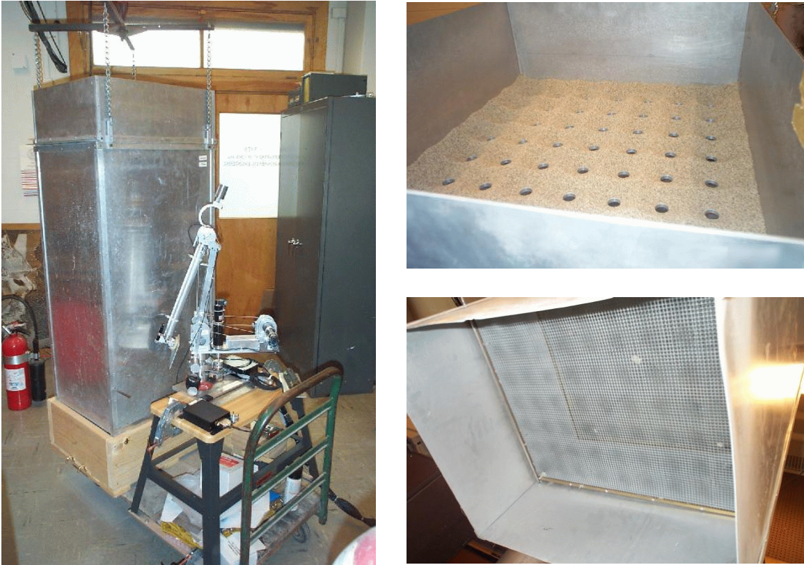
Figure 5-1: The raining assembly placed on top of sandbox for the deposition of uniform soil samples. The sandbox and manipulator are both mounted on a rolling cart for easy transport. The images to the right show the holes in the upper assembly and the screens in the lower assembly.
