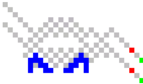
Figure 7-12: A CAM8 implementation of an identity gate (composed of two switch gates back to back) and a crossover. The shaded squares are the wires, visualized every other time step. The signals have exited the circuit at the right.
