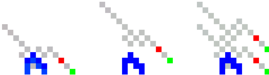
Figure 7-10: Three cases in the operation of a switch gate. Left: A = 0 , B = 1 . Center: A = 1 , B = 0 . Right: A = 1 , B = 1 . Particles are heavily shaded, cluster is black, and paths are lightly shaded. The path shading is only for every alternate time step, to make it simpler to resolve distinct paths by eye. The null case, A = 0 , B = 0 is omitted.
