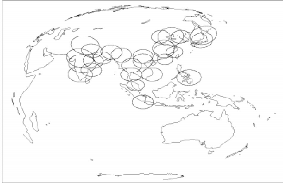
Figure 3.7: Asian Region GEO(3) Beam Pattern
