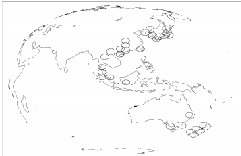
Figure 3.16: Pacific Rim 2 GEO(8) Beam Pattern
