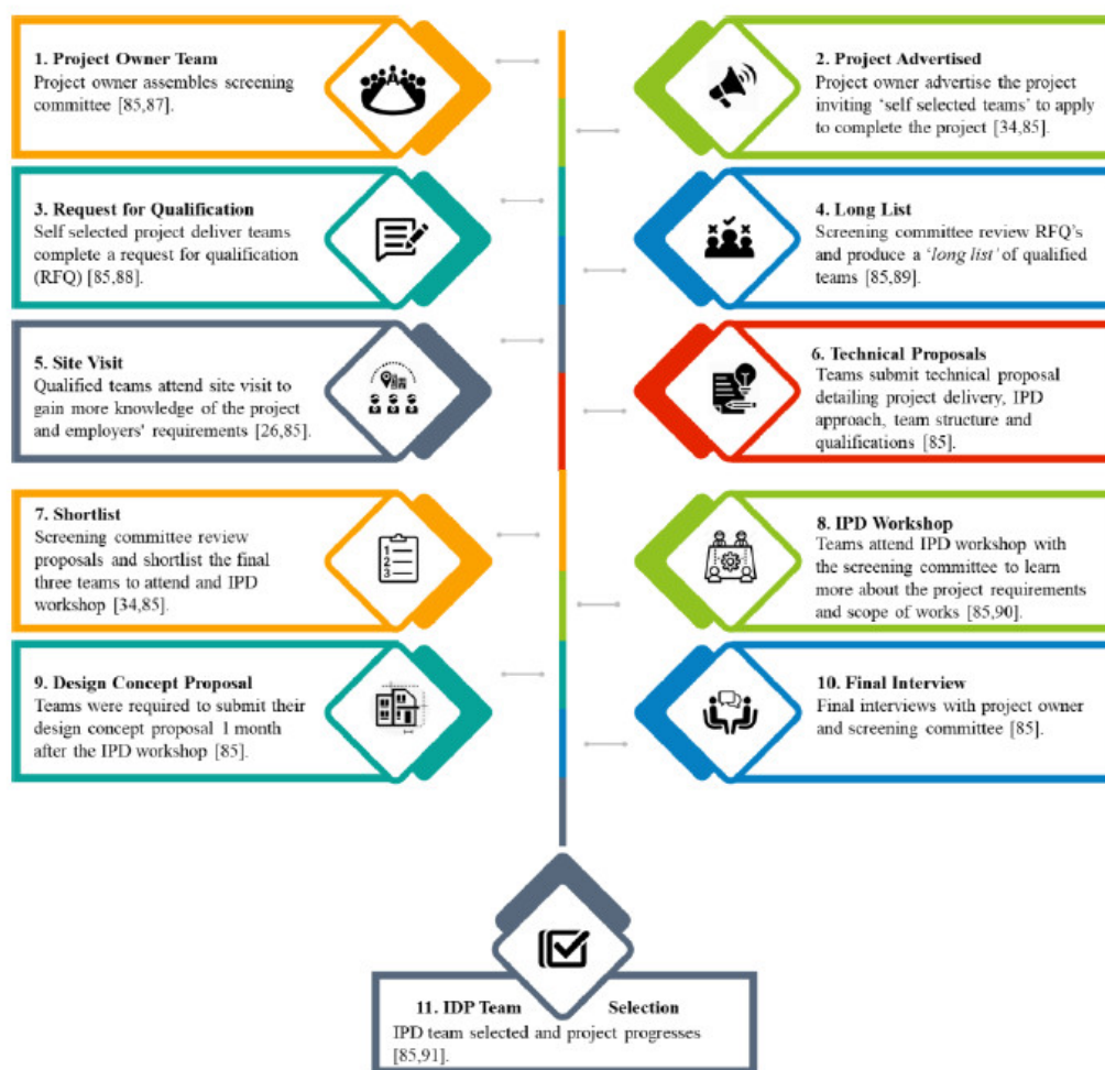
Figure 3. Integrated project delivery (IPD) selection process [26,34,85,87–91].
