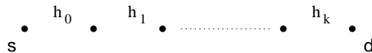
Figure 5-2: Case of n = 1 : h_i denotes the channel gain from relay i to relay i + 1 .
