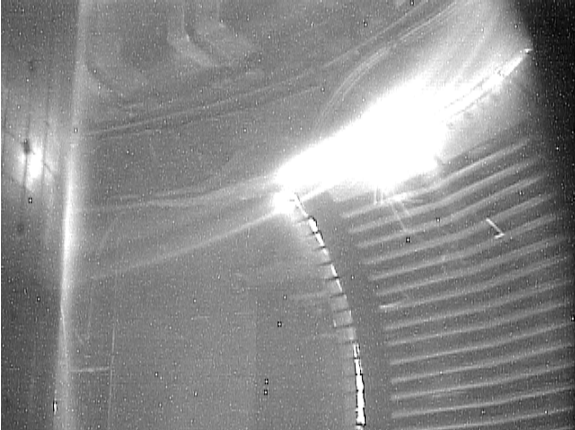
Figure 4-50: Recorded image from the visible imaging system showing an impurity injection from the RF antenna protection tiles. The central column can be seen on the left side of the view and the bars of the Faraday screen in-front of the RF antenna straps.
