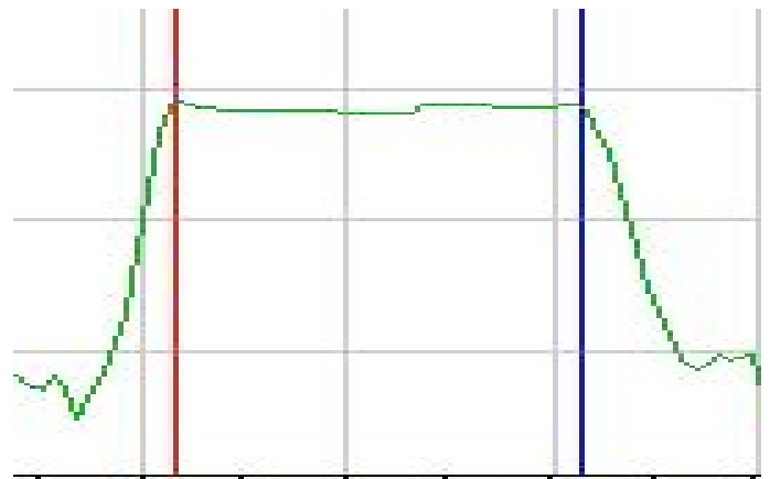
Figure 11 Width Profile for the "I" Feature from an AFM Scan. For this measurement the scan direction was actually along the long axis of the 'I', perpendicular to the width indicated.
