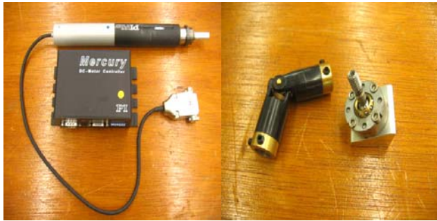
Fig. 9 The PI M-235.5DG actuator, Universal Joint and Spherical Joint.
