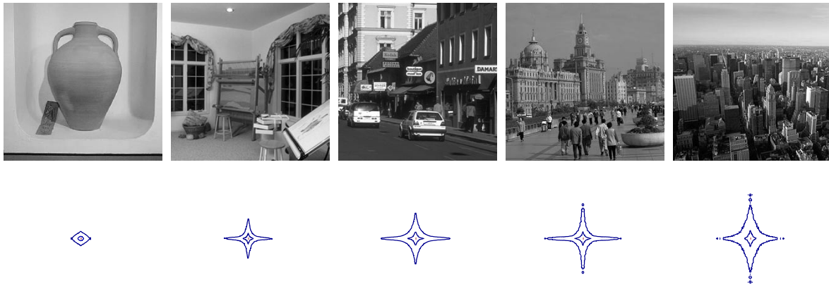
Fig. 6. Evolution of the global spectral signature of man-made structures with respect to the mean depth. Each signature is obtained from averaging over more than 300 pictures. The contour plots represent the 50% and the 80% of the energy of the spectral signatures.
