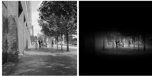
Figure 11. Person detection in large scenes where intrinsic information about faces and bodies may be highly impoverished. Left panel: a sample scene. Right panel: Results from a computational model for incorporating context in object detection tasks. Selection of image regions with high priors about people presence.
