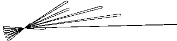
Figure 4. The trajectory of a simulated fly tracking a stationary target with nonlinear D_n(\psi) , and \Delta t = 0.01sec . The velocity is constant. After a transient bow-tie trajectory the model fly settles in one of the loops (the smallest one in the figure) with a periodic behavior (see inset). The same behavior is observed for different dt (from 0.1 to 0.001). Here, as in several of the following figures, the inset above the figure shows the error angle as a function of time. The ordinate is from -\pi to \pi , the abscissa starts at time 0.
