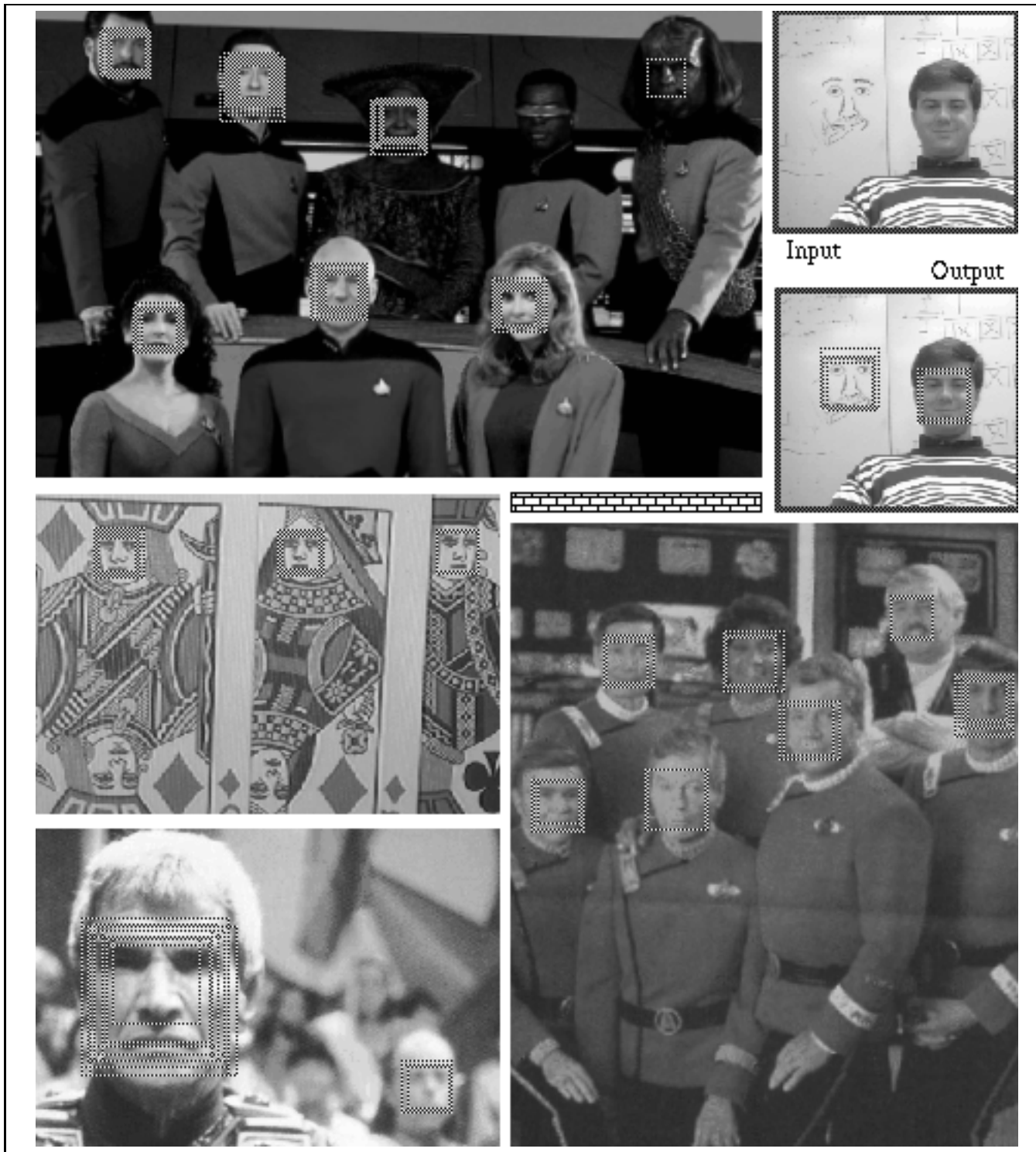
Figure 13: Some face detection results by our system. The upper left and bottom right images show that the system finds faces in complex scenes without making many false detects. The upper right image pair shows that the same system detects real faces and hand drawn faces equally well. The bottom left image shows the system working successfully at two very different scales. Notice that in the cards image, the system detects only the vertically oriented face patterns as it is meant to at this time.
