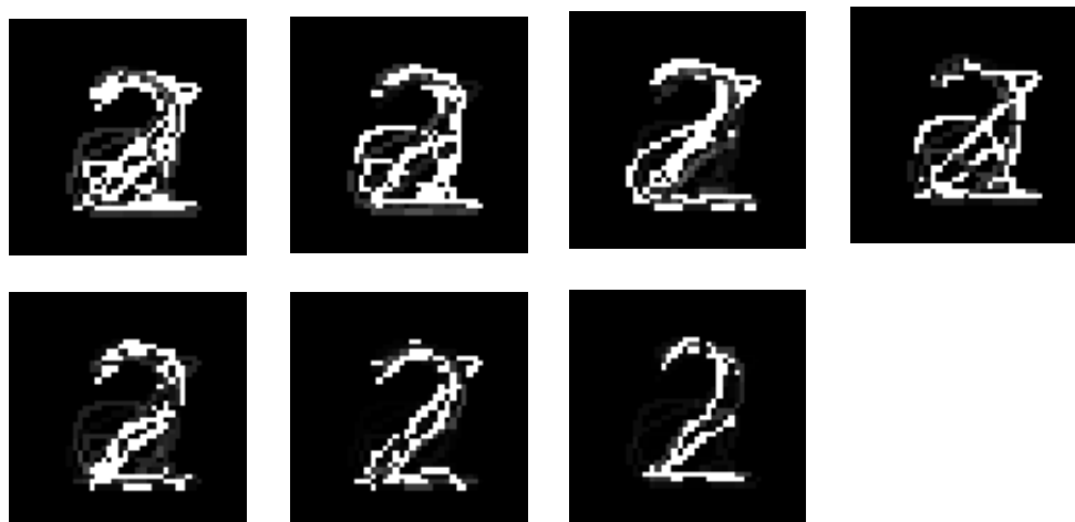
Figure 17: a) Mean image “2” found by averaging the prototype images of “2’s”. b) So-called eigenimages of “2’s”, that is eigenvectors computed from the set of images of prototype “2’s” (without using pixelwise correspondences).
