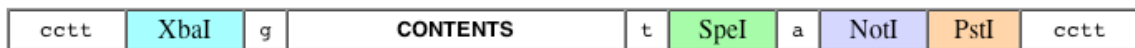
Fig. 2.3: A base part with the BioBrick prefix and suffix. The XbaI and PstI sites are used to cut the part when it is used in an assembly. There are a few extra bases inserted to separate the cut sites. [26]
