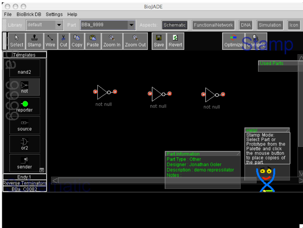
Figure 4.2: Schematic Design Mode. This figure shows three blank not gates being stamped out on the design. Note the context-sensitive help in the lower right corner.
