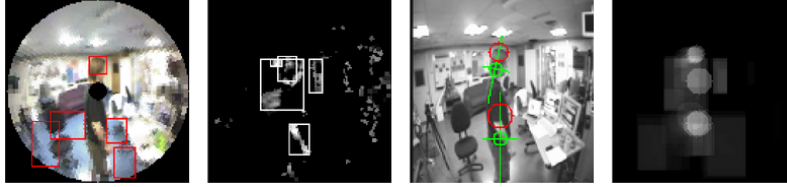
Figure 4.7: Saliency and attention processing while looking at a walking person. One frame each from the three saliency filters (vividness, skin tone, and motion) and the attention system is shown. The vividness filter picks out parts of the blue floor. The skin tone filter picks out the person’s arm and hair, a door, and the couch. The motion detector highlights picks out two targets on the person’s body. The regions chosen by the filters are weighted together by the attention mechanism, which favors the motion detector.
