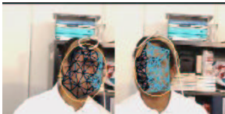
Figure 8.19: A visualization of surface coordinates on the mesh. The mesh has been colored here based on the sign of a surface coordinate, so that it appears as two halves locked onto either side of the face.
