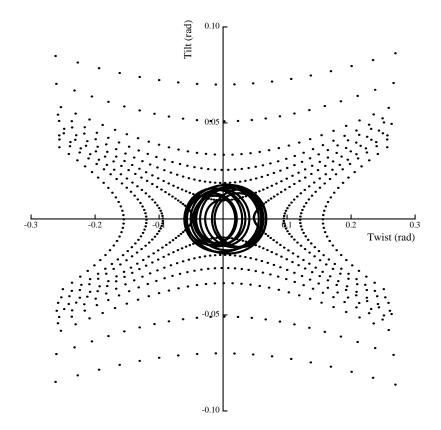
Figure 4-15: Tilt angles plotted as a function of twist angle for a non-linear dynamic simulation of the five d.o.f. passive model of the human. The simulated trajectory is superposed upon rigid body trajectories of the same model. This simulation was initialized with a tilt angle of 0.01 rad, zero twist angle and symmetric arm angle of 1.3 rad.
