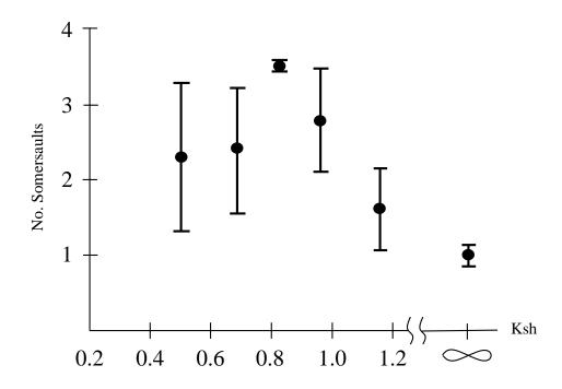
Figure 5-7: Plot of the average number of stable somersaults performed during twenty launches of the doll as a function of the shoulder spring constant,  $K_{sh}$ . The standard deviation is indicated by error bars. The data for the rigidly fixed arms is indicated by the infinite value of  $K_{sh}$ . The nominal arm angle was approximately 1.6 radians. The best value of  $K_{sh} = 0.82$  falls withing the range of stability predicted by theory as indicated in Figure 5-5.
