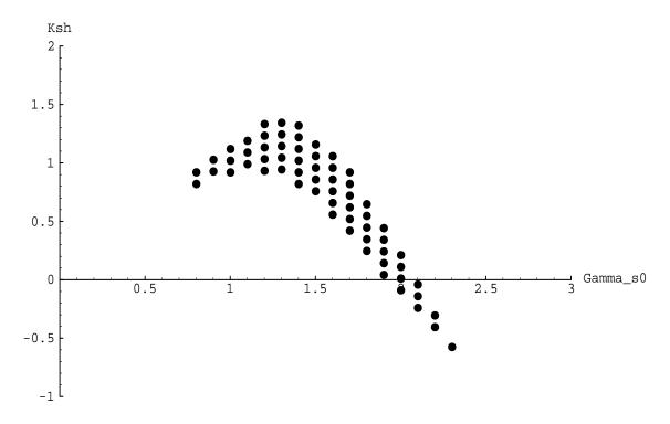
Figure 4-9: Each darkened point in this plot corresponds to a specific choice of  $K_{sh}$ and the nominal symmetric arm angle ( $\Gamma_{s0}$ ) that stabilize the full five d.o.f. linear system,  $b_{sh}/\dot{\Phi} = 0$ .
