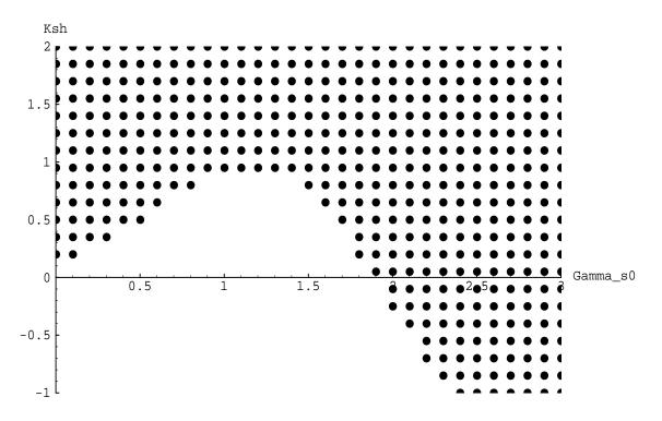
Figure 4-11: Each darkened point in this plot corresponds to a specific choice of  $K_{sh}$ and the nominal symmetric arm angle  $(\Gamma_{s0})$  that stabilize the two d.o.f. linear system of somersault and symmetric arm movement,  $b_{sh}/\dot{\Phi} = 0$ . Higher values of  $K_{sh}$  than are shown on this plot are suspected to also stabilize the system.
