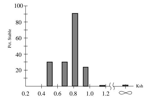
Figure 5-8: Plot of the percentage (of twenty) of completely stable dismounts as a function of the non-dimensional shoulder spring constant,  $K_{sh}$ . The two test conditions on the right side of the plot exhibited zero completely stable somersaults. The best value of  $K_{sh} = 0.82$  falls withing the range of stability predicted by theory as indicated in Figure 5-5.
