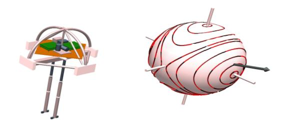
Figure 3-3: The somersault axis of the 3D Biped is coincident with the major principal axis of inertia. With the legs in the fully extended position, as shown here, the minor principal axis is the 'head-to-toe' axis.
