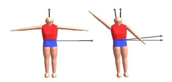
Figure 4-13: The orientation of the principal axes of inertia can be controlled with arm rotation. The tilt of the principal axes of the figure on the right is a result of body axis tilt due to airborne reorientation of the body plus principal axes tilt due to body asymmetry.
