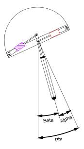
Figure 3-4: In order to maintain balance at landing the leg inclination angle,  $\beta$ , must be near the desired value.  $\beta$  is the angle the leg makes with the local vertical. It is a function of the the hip angle,  $\alpha$  and the body attitude,  $\Phi$ .
