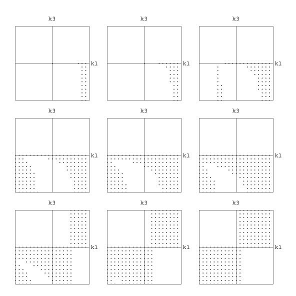
Figure 4-18: These plots show that  $1.0 \leq K_{sh} \leq 1.1$  produces the largest region of stable configurations for rotation about the middle principal axis for the "simplest model". Each dark point represents a stable configuration in  $k_1 - k_3$  space for rotation about a principal axis.  $kl_1 = -1$ ,  $I_{rel} = 0.1$  Each plot is for a different value of  $K_{sh}$ .  $K_{sh} = 0.0, 0.5, 0.8, 0.9, 1.0, 1.1, 1.2, 1.5$  and 2.0 for plots positioned from left to right and down the page.
