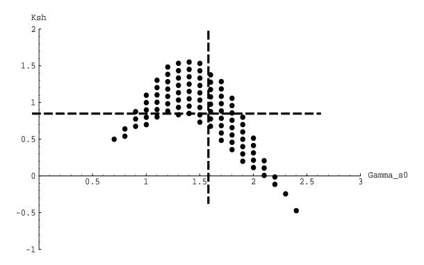
Figure 5-5: The points in this plot indicate the values of  $K_{sh}$  that theoretically will stabilize layout somersaults in the doll. The cross-hairs indicate the spring constant that best stabilized the doll during experiments.
