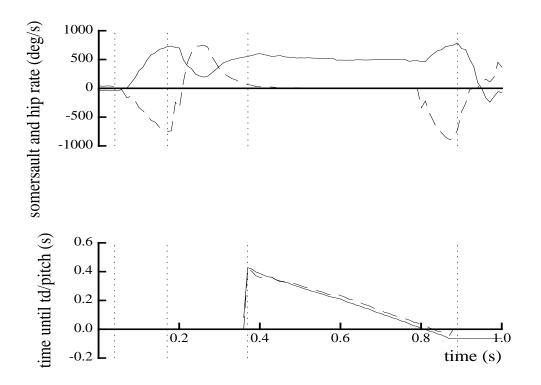
Figure 3-7: This somersault was over-rotating so the feet were swept forward at the end to track a desired foot position. Data shows absolute somersault rate (solid) and relative hip rate (dashed) and estimated time until touch down (solid) and estimated time until desired somersault attitude is achieved (dashed). Vertical lines indicate initiation of flip, lift-off, tuck servo initiation, and landing. Data file B92.181.4.
