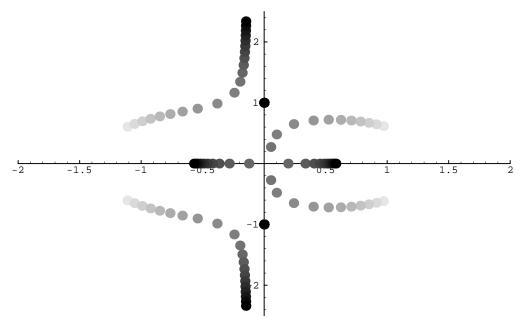
Figure 4-7: Root locus plot for the 3-by-3 subsystem of tilt, twist, and asymmetric arm movement.  $b_{sh}/\dot{\Phi} = 0.1$  and the nominal symmetric arm angle,  $\Gamma_{s0}$ , is 1.3 rad. Light dots indicate root locations for  $K_{sh} \approx -2.0$ . Dots get progressively darker as  $K_{sh}$  increases to 4.0.
