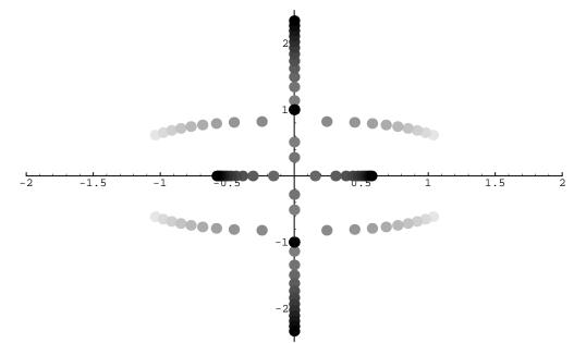
Figure 4-6: Root locus plot for the 3-by-3 subsystem of tilt, twist, and asymmetric arm movement.  $b_{sh}/\dot{\Phi} = 0.0$  and the nominal symmetric arm angle,  $\Gamma_{s0}$ , is 1.3 rad. Light dots indicate root locations for  $K_{sh} \approx -2.0$ . Dots get progressively darker as  $K_{sh}$  increases to 4.0.
