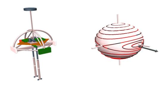
Figure 6-6: Spherical coordinate map of the tilt and twist Euler angle trajectories for the 3D Biped with 4 kg of weight added at a distance of 0.8 m above the hip.
