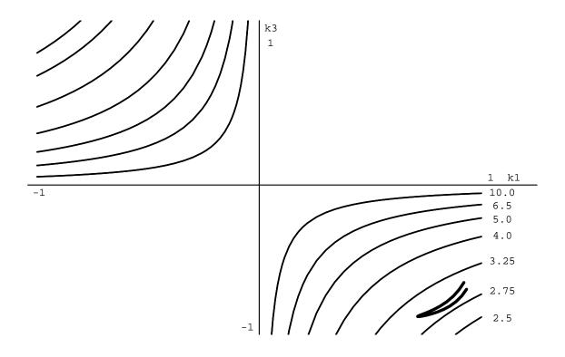
Figure 4-5: Rigid body stability diagram for Furrer's data. The dark lines show  $k_1$  and  $k_3$  for  $0 < \Gamma_{s0} < 3.0$ . The light lines are lines of constant  $\Phi$ , the change in somersault angle required for the unstable rigid body mode to grow by a factor of ten. The plot shows that the human form is relatively unstable in the rigid body sense.
