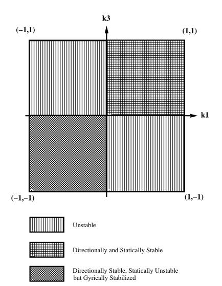
Figure 2-3: Stability diagram for the simple spin solutions of a rigid body. Rigid body rotational stability depends only upon the two non-dimensional inertia ratios  $k_1$  and  $k_3$ . We assume the body is rotating about the principal axis corresponding to  $I_2$  for this diagram.
