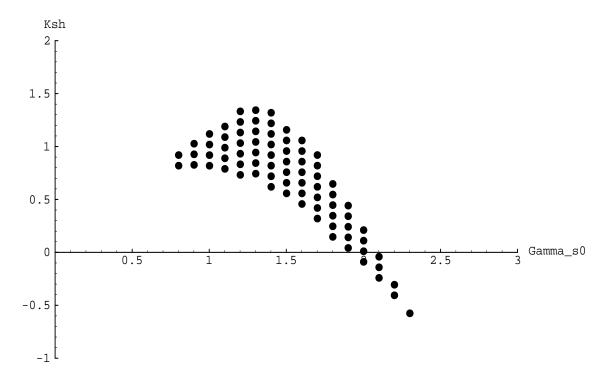
Figure 4-10: Each darkened point in this plot corresponds to a specific choice of  $K_{sh}$  and the nominal symmetric arm angle  $(\Gamma_{s0})$  that stabilize the three d.o.f. linear system of tilt, twist, and asymmetric arm movement,  $b_{sh}/\dot{\Phi} = 0$ .
