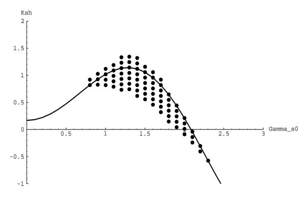
Figure 4-17: Plot of the stabilizing  $K_{sh}$  for a the 3-by-3 subsystem of the human model. The solid curve shows the value of  $K_{sh}$  that will exactly cancel the spring term due to centrifugal forces on the arm.
