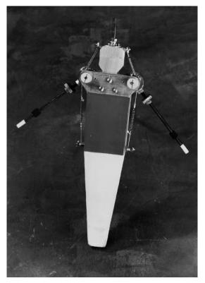
Figure 1-3: Photograph of the mechanical doll used for experiments with layout somersaults. The doll could consistently perform stable, triple layout somersaults.
