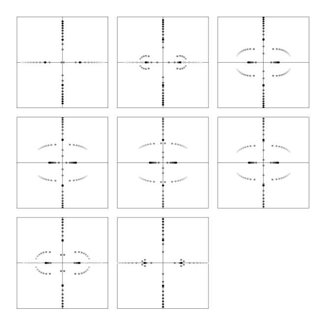
Figure 4-8: Root loci for the 3-by-3 subsystem of tilt, twist, and asymmetric arm movement as the nominal symmetric arm angle,  $\Gamma_{s0}$ , is varied between 0.0 (top left) and 2.8 rad (bottom center),  $b_{sh} = 0$ ,  $-2.0 < K_{sh} < 4.0$ .
