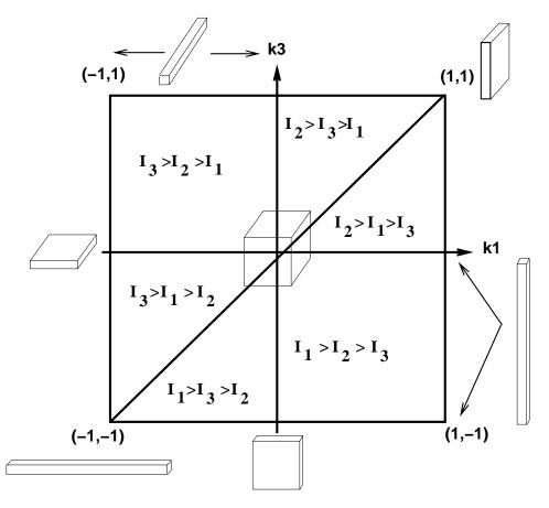
Figure 2-2: The inertia ratio diagram shows how  $k_1$  and  $k_3$  depend upon the relative value of the principal inertias.  $k_1 = \frac{I_2 - I_3}{I_1}$ ,  $k_3 = \frac{I_2 - I_1}{I_3}$ . The different rectangular prisms located near the axes and corners of the diagram indicate an example shape that would correspond to the local inertia ratios.
