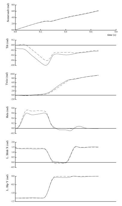
Figure 6-5: Simulation data from a 1 1/2 twisting somersault with  $\omega_n = 30, \Theta_0 =$ -0.1, and  $\Psi_0 = -0.1$  are shown with solid lines. The desired values of the body attitude and joint angles are shown with dashed lines. Joint angles incur significant tracking errors but the landing attitude closely follows that of the nominal maneuver. (The traces stop at the landing time.)
