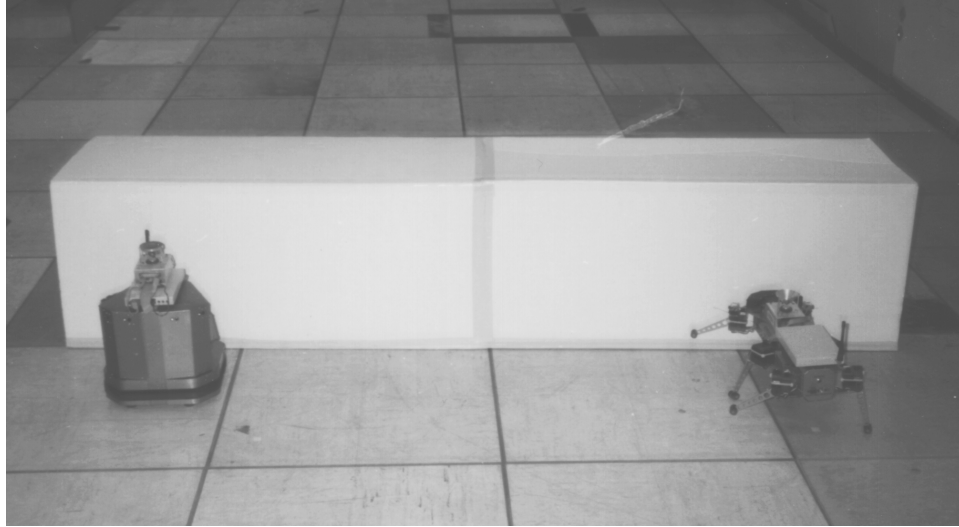
Figure 6-5: Adaptivity due to heterogeneity. In this second experiment, I again seize one of the R-2 robots, but this time I replace it with Genghis-II. Since Genghis-II cannot push as powerfully as an R-2, the remaining R-2 robot adapts its actions by pushing less frequently.
