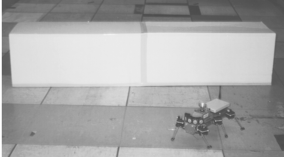
Figure 6-6: Response to robot failure. At the end of the second experiment, I seize the remaining R-2 robot, leaving Genghis-II alone to perform the demonstration. Since Genghis-II cannot complete the demonstration on its own, it activates its go-home behavior set.
