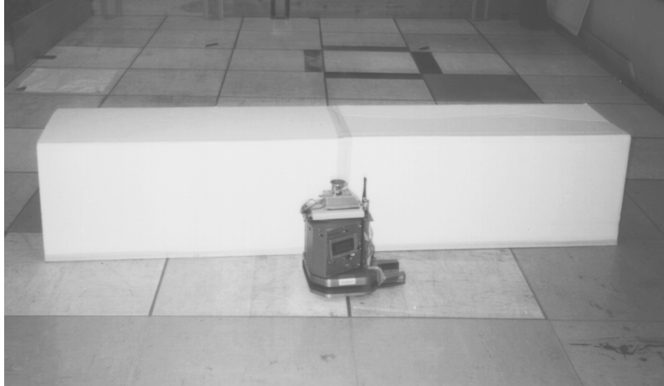
Figure 6-4: Fault tolerant action selection. In this first experiment, I seize one of the R-2 robots and turn it off. This causes the remaining R-2 robot to have to perform both tasks of the box pushing demonstration: pushing at the right end of the box, and pushing at the left end of the box.
