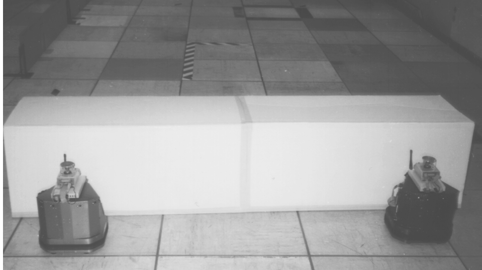
Figure 6-3: The beginning of the box pushing demonstration. Two R-2s are pushing the box across the room.
