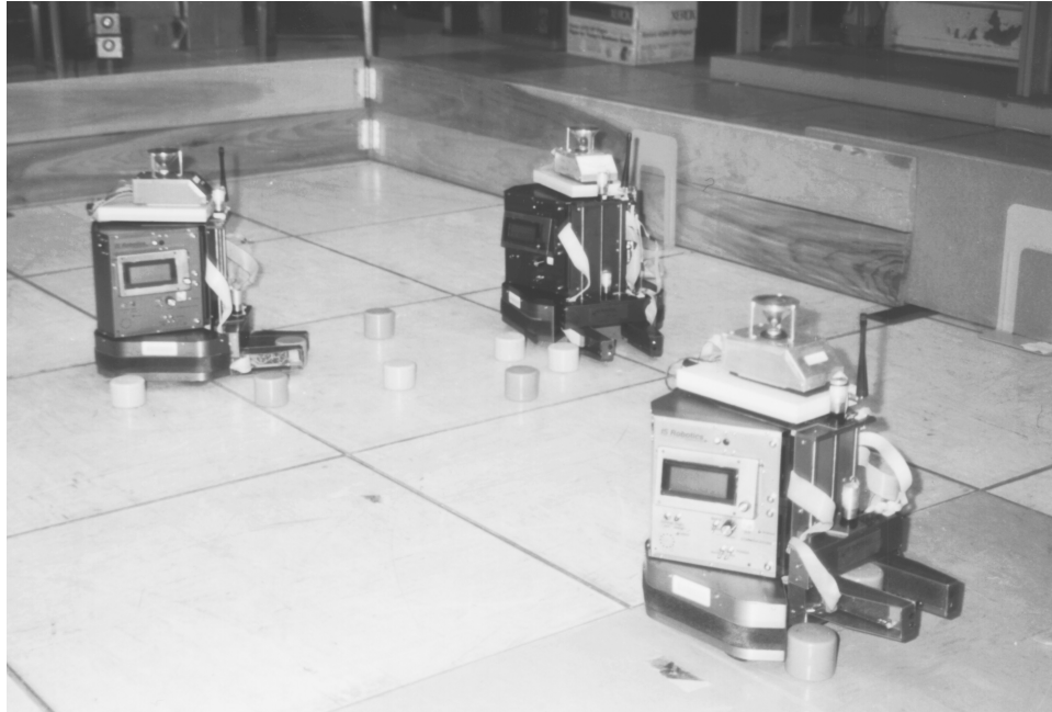
Figure 3-15: The rightmost R-2 in this photograph has just grasped a spill object and is taking it to the goal location. Note the additional puck caught in the cavity below the gripper, which allows this robot to transport more than one spill object on this trip.
