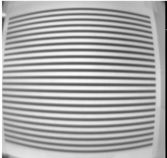
Figure 3: Typical images of vertical and horizontal bars taken with the Chinon camera and a wide angle lens. These images were used to calibrate the radial distortion parameters with the 'plumb line' method
