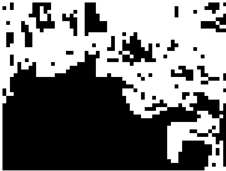
Figure 1.2: The pixels with significant texture. Pixels marked in white differ from their neighbors above and to the right by total of at least 15 grey levels out of a possible 510. Pixels marked in black differ by less than 15 grey levels. The image was first smoothed with a 3 \times 3 filter to remove camera noise. Note that the floor is uniformly black.
