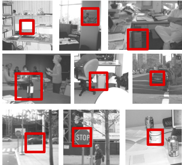
Fig. 10. Examples of correct detections of several object detectors trained jointly (screen, poster, cpu, bottle, trash, car frontal, car side, stop sign, mug).
