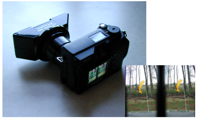
Figure 3: The apparatus for taking synchronized stereo image sequences: Olympus Camedia C-3040 camera, and a Pentax stereo adapter (connected using a Kenco 41mm - 52mm adapter ring). The digital camera can take 5 full-resolution shots in a row at 1/3 second intervals. The L/R split-screen image is visible in this photo on the camera’s LCD display. Insert: a typical split-screen image recorded by the camera.
