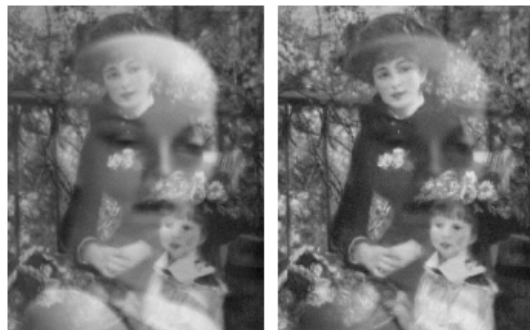
Figure 1: Renoir’s On the Terrace with a reflection of Sheila photographed through a linear polarizer at orthogonal orientations, maximizing and minimizing the reflection.
