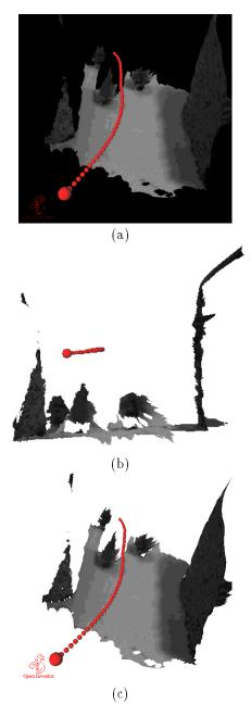
Figure 2: (a,b,c) Show 3D renderings of the scene. Very distant surfaces have been removed. The spheres show the motion of the stereo rig in the whole sequence. The large sphere is the the location of the camera when this image was taken. Not in view (b) that the ground plane is correctly found to be flat at the the two cork walls are at right angles to the it.
