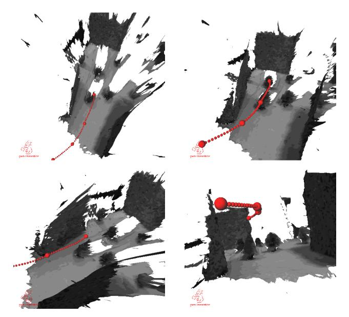
Figure 8: Euclidean reconstruction of the extended scene created by aligning four separate reconstructions into one coordinate system using the recovered camera motion. The small spheres show the camera path. The large spheres show the camera positions of the four Euclidean reconstructions.
