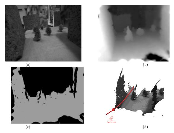
Figure 5: (a) The 14th image in the sequence. (b) The depth map. (c) The mask. We do not render surfaces that are far from the camera or where the surface is facing the camera with a sharp angle. (d) rendering of the surfaces.
