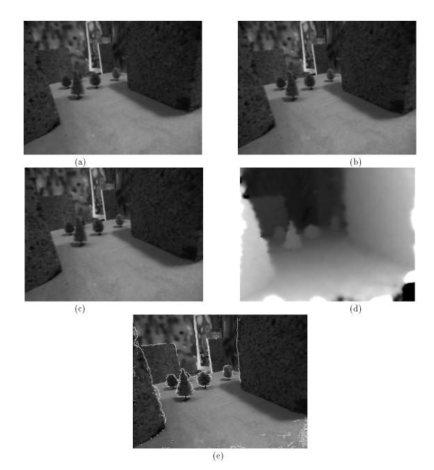
Figure 1: The three input images (a,b,c). Image (a) and (c) are the first stereo pair in the sequence with the cameras displaced vertically. Image (b) is the image from camera (a) taken at the next time instance. (d) the estimated depth map.. (e) shows the results of a Canny edge detector on the depth map. This identifies occluding contours.
