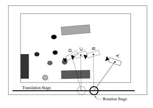
Figure 3: Schematic overhead view of the 'fly-through' scene indicating the three cork blocks, 6 model tree (circles) and the motion stage (not to scale). The camera arm is rotated  $45^{\circ}$  in  $1.5^{\circ}$  steps from position A to position B. The arm then translates in twelve 1cm steps to position C. Then it Rotates through  $12^{\circ}$  to position D.
