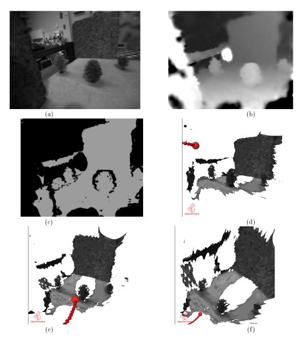
Figure 7: (a) The 49th image in the sequence. (b) The depth map. (c) The mask. (d), (e), (f) 3D renderings of the surfaces. In this view a bit of the translation stage can be seen (top left quadrant).
