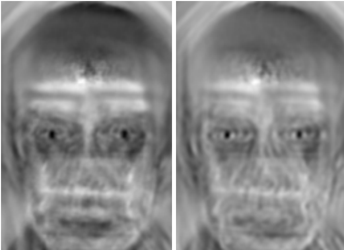
Figure 7: The output of the correlation with an SDF computed using the spectral envelope of 20 training images as whitening preprocessing. Left: the normal SDF (20 examples). Right: a least square SDF with 6 templates (20 examples). The darker the image the higher the corresponding value. The least square SDF exhibits a sharper response using the same whitening filter.
