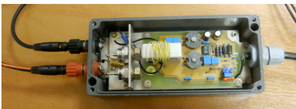
Fig. 2. The Hall sensor with a \pm 15 V output range
