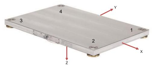
Figure 17 Kistler force platform with four force sensors, and the directional axes of measurement
