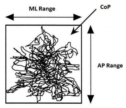
Figure 18 Visual representation of CoP path, and directional specific Range (anterior-posterior [AP] and medial--lateral [ML]) variables during standing balance
