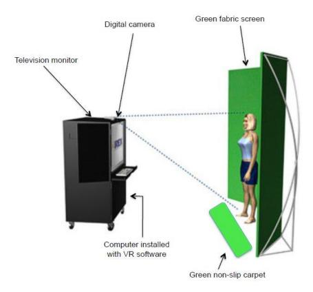
Figure 6 The IREX<sup>™</sup> system – Setup (GestureTek<sup>™</sup> Health 2008)
