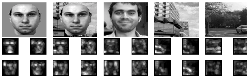
Figure 2.2: Typical stimuli and associated responses of the C1 complex cells (4 orientations). Top: Sample synthetic face , cluttered face, real face, non-faces. Bottom: The corresponding C1 activations to those images. Each of the four subfigures in the C1 activation figures maps to the four bar orientations (clockwise from top left: 0, 45, 135, 90 degrees). For simplicity, only the response at one scale is displayed. Note that an individual C1 cell is not particularly selective either to face or to non-face stimuli.
