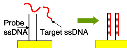
Fig. 5 Surface reaction of DNA hybridization occurs in DNA microarrays.
