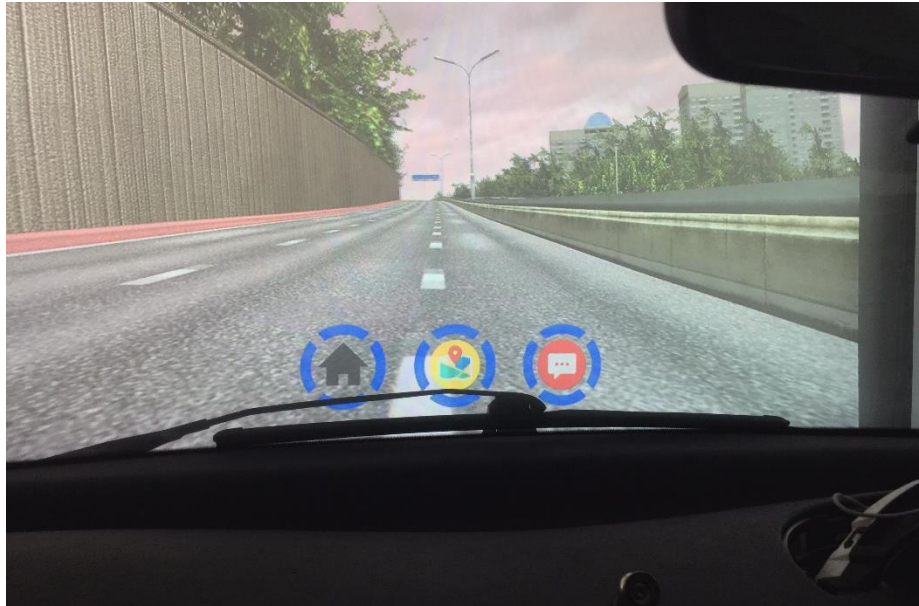
Fig. 1. Case 1: Driver's AR HUD and gesture recognition for controlling infotainment sources.
