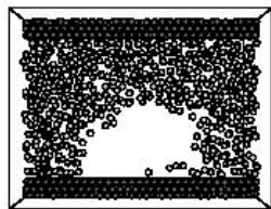
Figure 3: MD simulation of Argon bubble nucleation between parallel plates at 100K [25]. The bubble is the void region.
