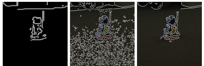
Fig. 6. From left to right: boundary detection with our algorithm, with the default Canny edge detector, and with a hand-tuned Canny edge detector.
