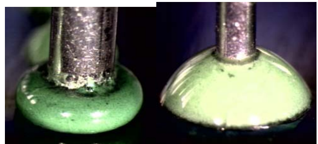
Fig. 9. Photographs of a glass bond between Kovar tubes and silicon test devices. The Kovar tubes are approximately 1 mm in diameter. Note that in the right hand photograph good wetting is achieved of the glass to silicon. This is preferable for the mechanical performance of the device. The wetting
