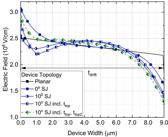
Fig. 7. Electric field distribution, at the onset of  $V_{BD}$ , through the center of the n-drift region of SJ structures with varying degrees of  $\alpha$ , in reference to a planar SBD optimized to 2.1 kV.
