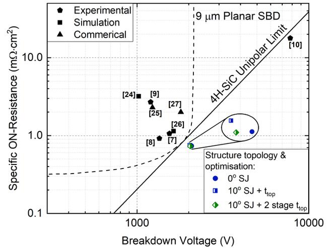
Fig. 14. SJ devices with comparable  $R_{ON,SP}$  [7]–[10], [24]–[27] plotted against the 1-D limit of 4H-SiC and an ideal  $9\text{-}\mu\text{m}$  planar device. The graph includes the optimized device from this study.
