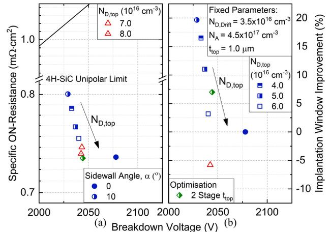
Fig. 6. Effect of a highly doped surface region with a fixed depth,  $t_{top} = 1.0 \mu\text{m}$ , and varied doping on (a)  $R_{ON,SP}$  and (b) implantation window (at 80% of  $V_{BD,PEAK}$ ), shown as the relative improvement in comparison to the 0° SJ structure.
