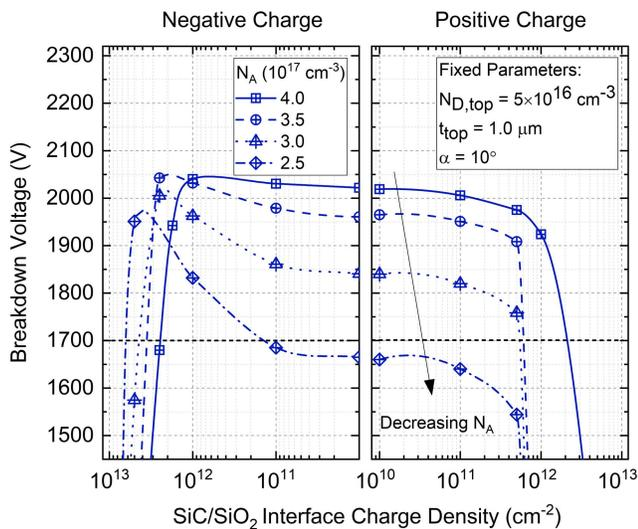
Fig. 10. Influence of SiC/SiO<sub>2</sub> interface charge density on  $V_{BD}$ .
