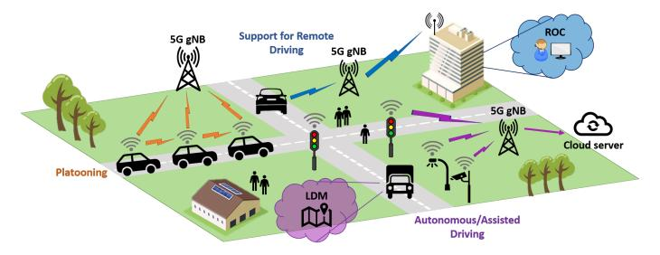
Fig. 1. High-level overview of the advanced use-cases expected to be supported by 5G V2X.
