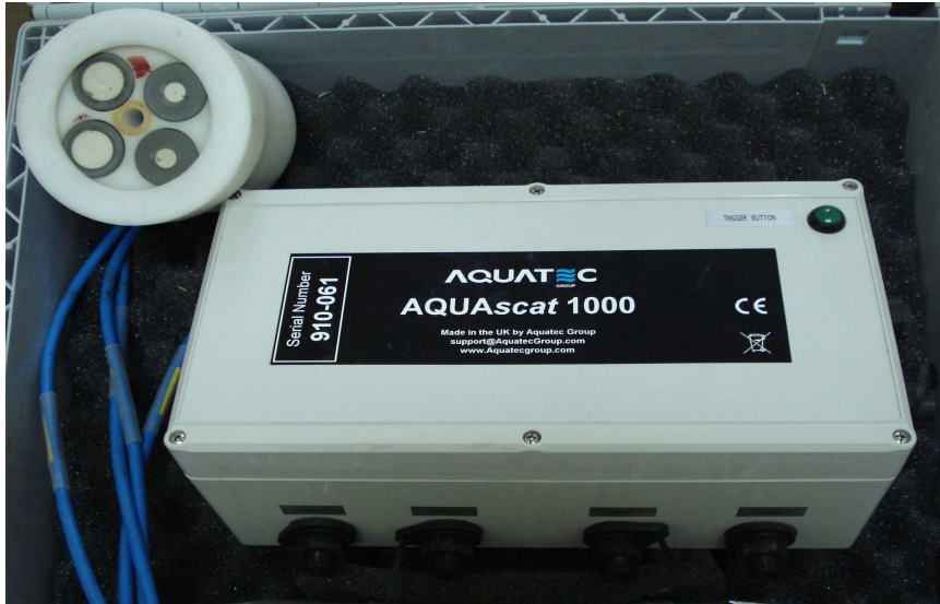
Fig 1. An acoustic backscatter system (AQUAscat 1000) with transducers
