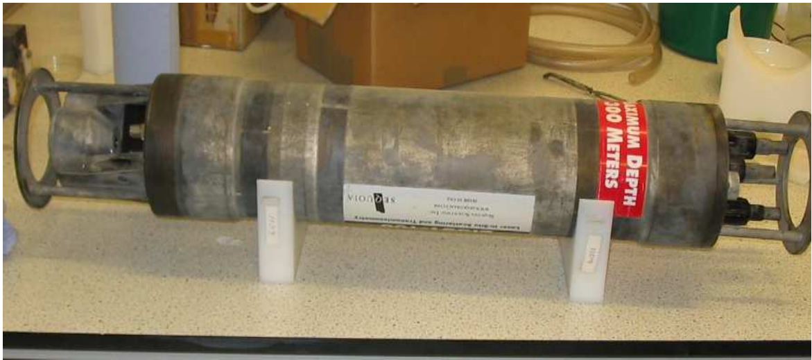
Fig. 2 . The LISST-100 devices for sediment measurement with laser scattering technique
