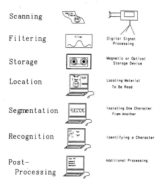
Figure 2: Key steps in automated reading
