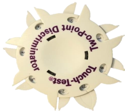
Figure 2.7. Two-point discrimination touch test. Point spacing numbers correspond to mm of the two distinct points.
