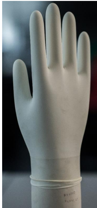
Figure 2.5. Glove formed on porcelain mould.
