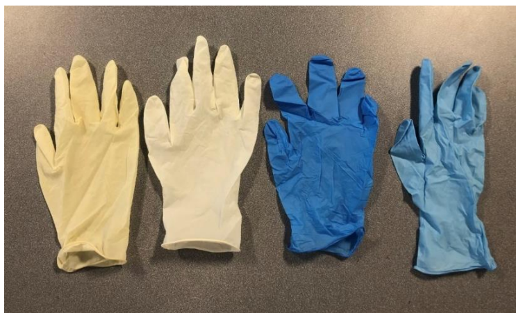
Figure 4.1. Glove selection used in this study. From left to right; chlorinated NRL; polymer coated NRL; chlorinated NBR; and polymer coated NBR.
