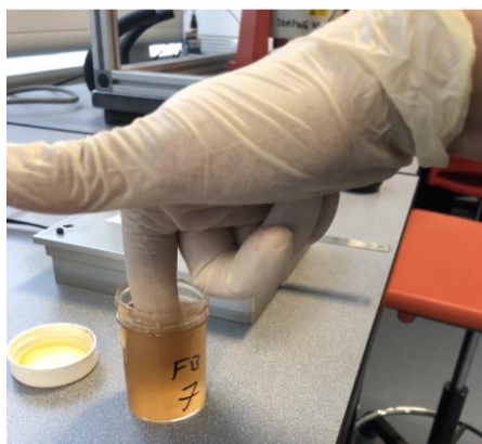
Figure 9.2. Application of solutions to the glove materials
