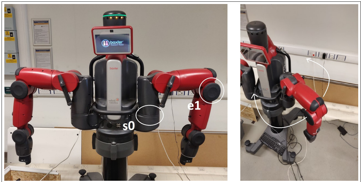
Figure 42: A pair of images of the Baxter Robot. The left image shows the robot, the controlled joint ( s_0 ) and the location that was being controlled ( e_1 ). The control system applies torque to the joint s_0 , which rotates the arm in the XZ plane. This moves the e_1 joint around Baxter's body. The control system is controlling the relative angle of the e_1 joint with respect to Baxter. The right image visualises the effect of applying force to the s_0 joint to demonstrate the domain of the task.
