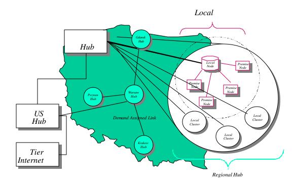
The ISP connects to the network via a Frame Relay or ATM depending on the carrier, which circumvents the modem pools. This is a higher speed, continuous time, and lower cost means of interconnection. The Internet Network allows for any user to have remote high speed access to the Internet at speeds up to 100 Mbps. This system provides for the most cost effective interconnection alternative that is available. There is a hub location that interconnects into the Internet Service Provider, ISP.
