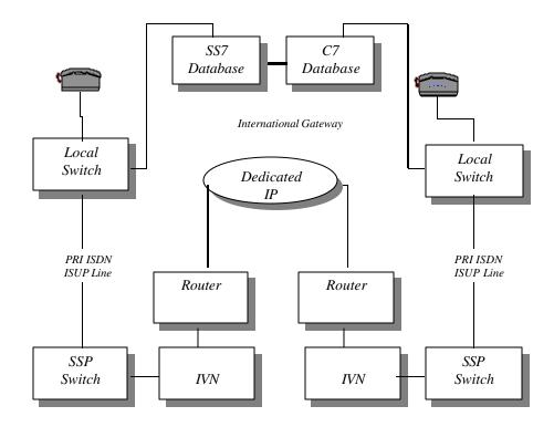
The basic system building block for services is the IP Voice Node (IVN), shown below:
