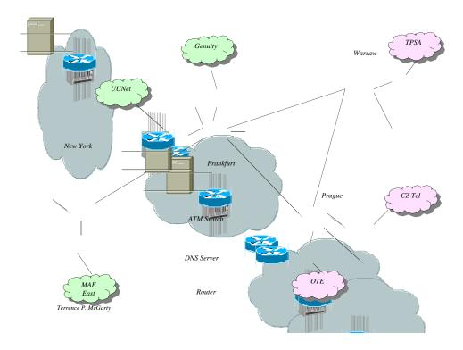
The overall architecture of the MAE Europe construct is shown below. It consists of NAPs which are interconnected as a distributed single entity. These NAPs then interface with other NAPs and MAE East and West, as may be required.
