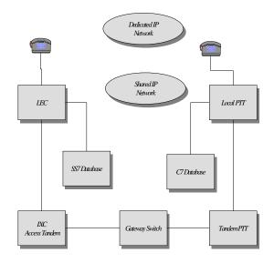
The next variant is with the use of an IP carrier. We have depicted two different types. The first is a decocted backbone IP network and the second is a shared IP backbone network. The shared is what we typically call the open Internet whereas the dedicated is the closed user Internet, sometimes called an Intranet, although this is generally reserved for a completely closed user group.
