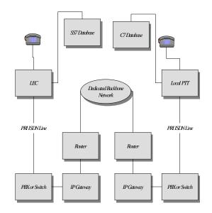
In this Figure we depict the Routers, the clear channel backbone network as well as any IP gateways. However we also depict a PBX or switch for interconnect to the LEC or PTT. This may or may not be necessary.
